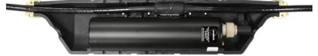
Magnetometer sensor - shown installed on the array cable with protective shell open
